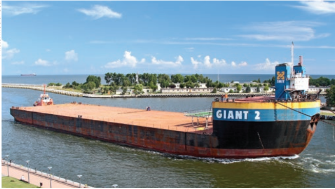
Newly purchased by Remontowa S.A. heavy lift barge Giant 2 has become a new floating dock for ships and offshore platforms.
