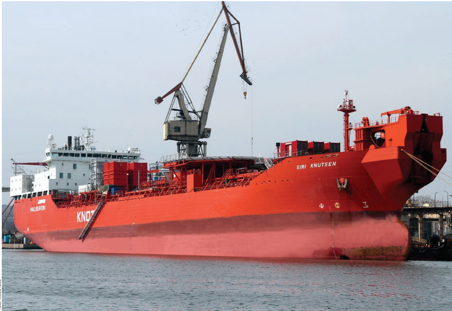
Siri Knutsen converted at Remontowa SA into a well stimulation vessel.
