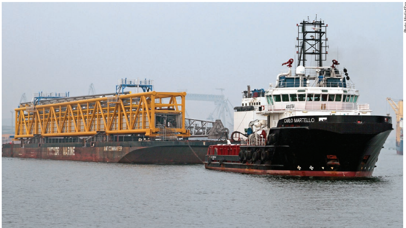
Transport bridge and flare tower from Vistal for Eldfisk platforms complex expansion project.
