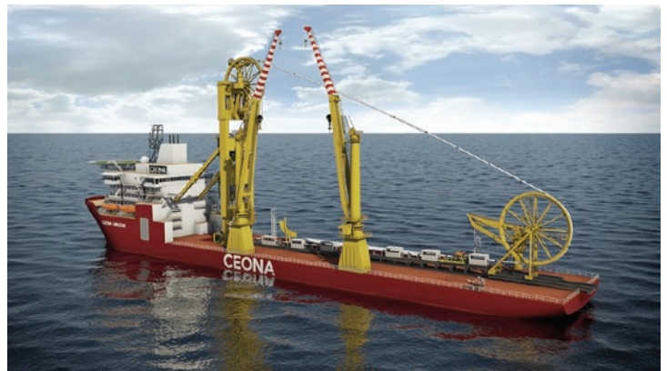
The ship will be required to lay fixed and flexible pipes on the seabed in water as deep as 3000 metres.
